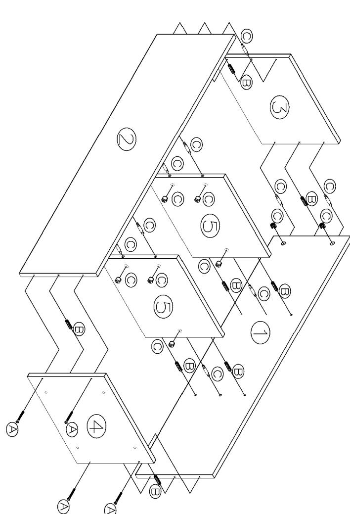
**DIAGRAMA 1: DETALLE MONTAJE DE PUERTAS**
